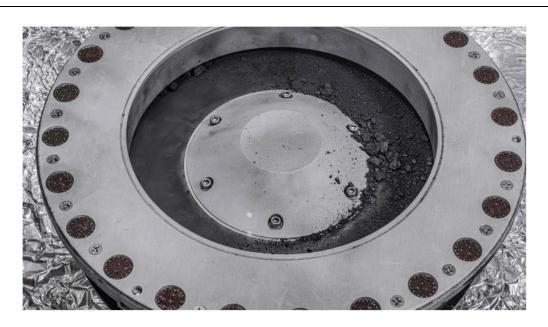
A view of the outside of the OSIRIS-REx sample collector. Sample material from asteroid Bennu can be seen on the middle right. Scientists have found evidence of both carbon and water in initial analysis of this material. The bulk of the sample is located inside.
