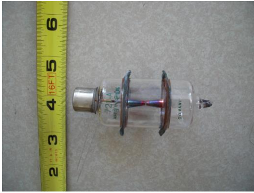
(Fig. 9, a Sylvania 721A, a type of radar T/R switch From the CHRS collections, photo Bart Lee)
