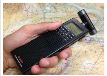
Countycomm GP5/SSB - the latest and best portable hand held HF SSB receiver in the world. Fully software defined using the SiLabs chip. Has software defined product detector. 1000 memories.
