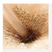
The circuits' filamentary serpentine shape allows them to bend, twist, scrunch and stretch while maintaining functionality. | Photo courtesy John Rogers
