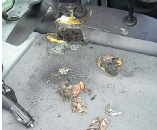
Figure 2: A cell phone with a no-brand battery that vented with flame while charging in the back of a car
