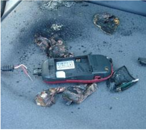
Figure 2: A cell phone with a no-brand battery that vented with flame while charging in the back of a car
