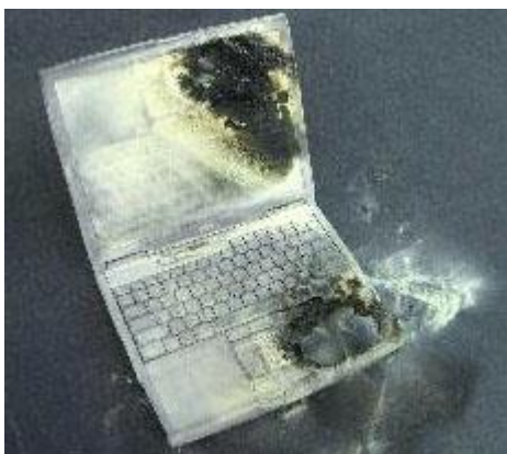
Figure 1: Lithium-ion battery damages a laptop.
