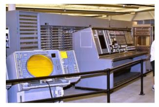
This computer is all tubes and was originally designed to track incoming Soviet Union bombers during the cold war. Unfortunately by time the computer was finished, ICBM's were the state of the art and this machine could not track fast incoming missiles. This computer was later used to track domestic aircrafts. It was still in service as late as 1984.
