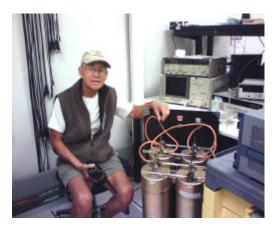
Here is George W6BUR in my lab in Sunnyvale where we retuned the duplexer for the repeater. The instrument in the background is an Agilent 8753D 6 GHz network analyzer. This is an essential instrument in tuning duplexers taking the guess work out of using old tracking generators and spectrum analyzers. The repeater, unfortunately still has this audio problem which we are trying to hunt down.
