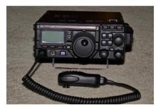
The grand prize will be a Yaesu FT897. This is an all mode, all band radio. 100 watts out on HF, 50 watts on VHF and 25 watts on UHF. Built in keyer, general coverage receiver, scanner, etc. It can be operated as a portable with built in battery packs, a base or mobile.
