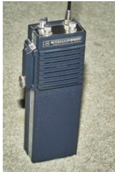
2. 6 channel version of the HT220. It uses an extra piggyback board for the extra channels and is about twice as thick as the slimline.
