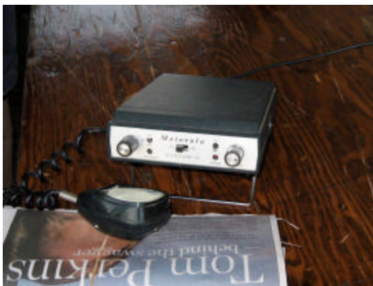
Our workhorse was a Motorola Sycom 10. This a fully synthesized radio with self contained batteries that will run for 40 hours in emergencies.
