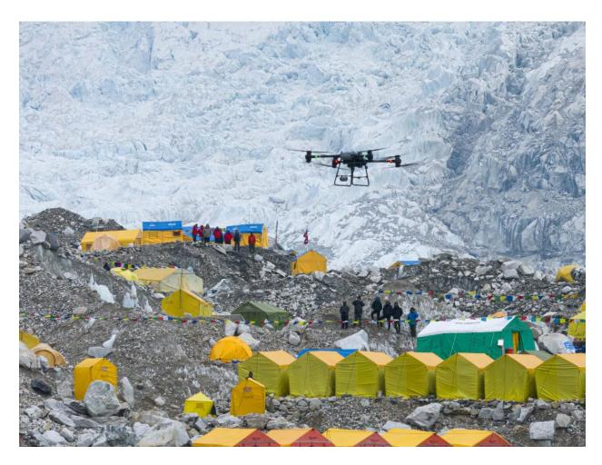
Before undertaking delivery flights, DJI engineers considered the extreme environmental challenges of Everest, including temperatures ranging between -15°C (59°F) to 5°C (41°F), wind speeds up to 15m/s (33.55 mph), and high altitudes over 6,000m AS (19,898 feet).
