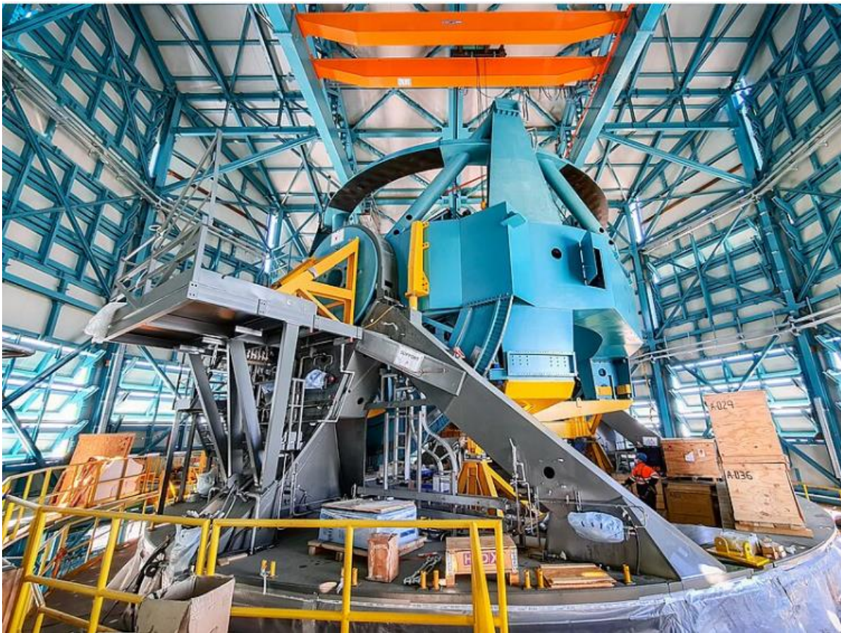
Telescope Mount Assembly of the 8.4-meter Simonyi Survey Telescope
