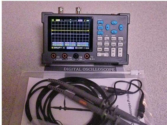
DSO03D12 120 MHz dual trace scope with probes - features a built in DVM , Signal generator, and FFT spectrum analyzer.
