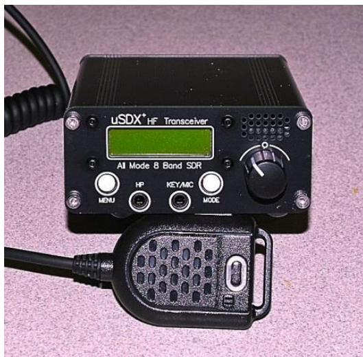
uSDX+ - QRP HF transceiver - Covers 160-6 meters – SSB, CW, digital QRP transceiver. 5 watts CW – 10 watt SSB. Built in CW decoder, full DSP noise reduction. Complete with 4000 MaH LiOn battery, AC adapter/charger, Speaker/microphone
