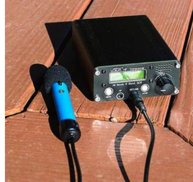
uSDX+ portable radio and microphone with a built-in light weight 4 Amp hr Lion battery.
