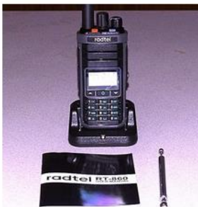
Radtel RT-860 1024 channels 2m/1.25m/70cm transceiver; full HF all mode receiver; preprogrammed with local channels
