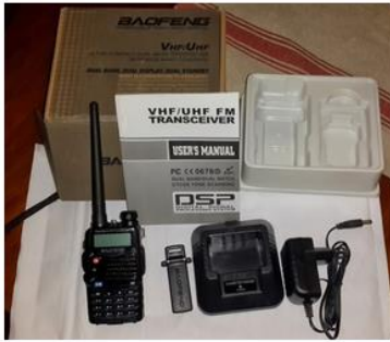
BaoFeng UV-5R x2 Dual Band VHF/UHF HT, 136-174MHz VHF (5W TX), 420-520MHz (4W TX), FM Broadcast, 128 channel memory, 1.8-Ah Li-Ion battery, drop-in smart charger
