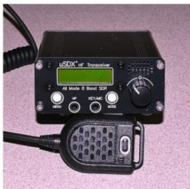
uSDX+ QRP HF transceiver Covers 160-6 meters – SSB, CW, digital QRP transceiver. 5 watts CW – 10 watt SSB. Built in CW decoder, full DSP noise reduction. Complete Description of prize.
