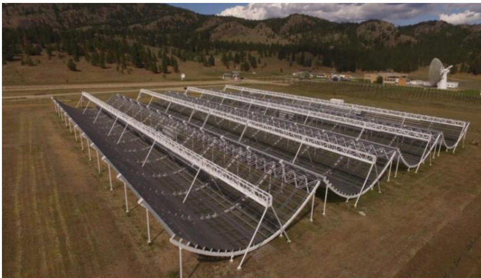
The CHIME array outside Penticton, British Columbia, is a novel radio telescope that has no moving parts. Designed to map hydrogen gas in the universe, it is also ideal for detecting fast radio bursts. Courtesy of the CHIME collaboration
