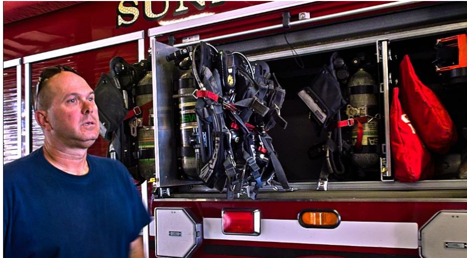
Jeff, 30 year with the Fire/Police Department show their carbon fiber SCBA breathing gear that is pressured with 4500 psi of air.
