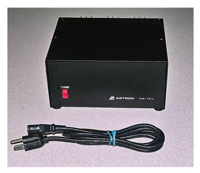
**Astron 12** - 12A linear power supply. Less than 5mV ripple even at full load.
