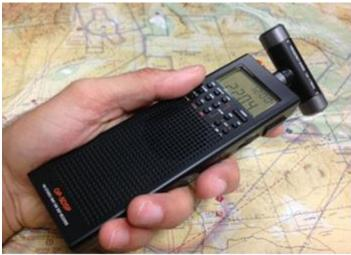
LW frequency: 150 - 522 kHz AM/SSB/CW
