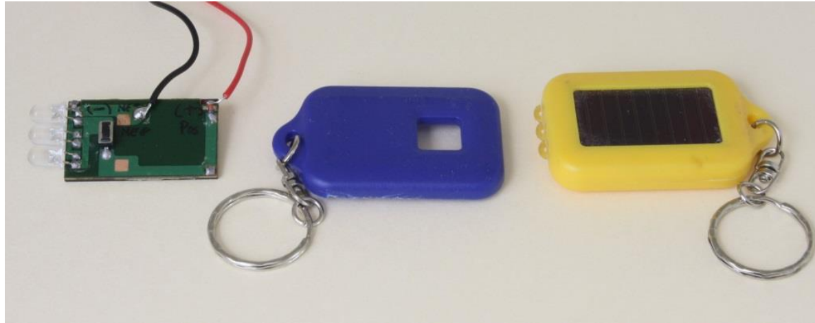
3 LED solar rechargeable flashlight disassembled.
