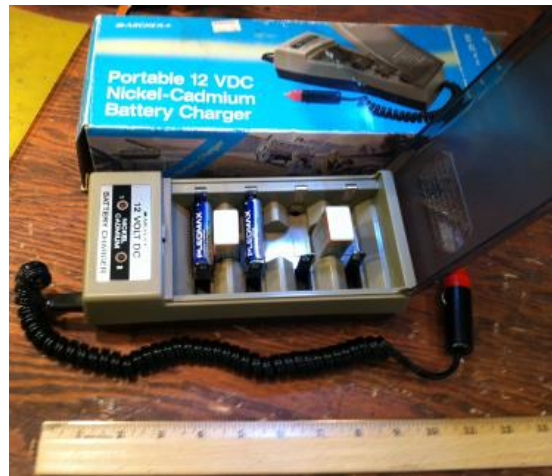
Bart Lee -K6VK's Ni-Cad battery charger for 12 volts. Photo by Bart Lee
