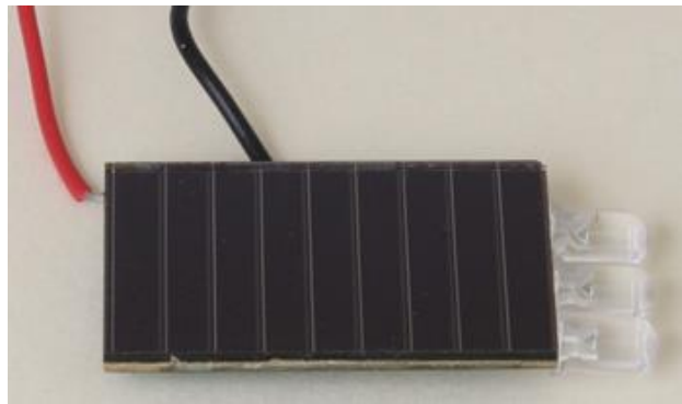
Flip side of circuit board with solar panel attached
