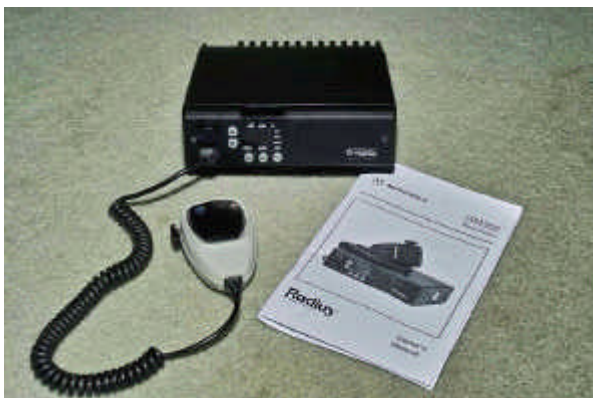
A typical MURS base station would be a Motorola GM300. Its output must be reduced to 2 watts for this service.
