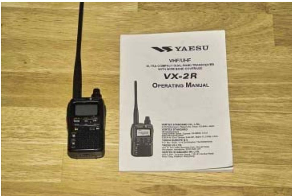
Yaesu VX2 - This is a great portable hand held with 1000 memories and includes the LiOn battery. This is the export model (you know what I mean). It receives AM/FM broadcast, SW broadcast, two way radio FM (30KHz), narrowband FM (12.5 KHz). It transmits VHF and UHF conventional and the new narrow band format. This is a great example of great things come in small packages.
